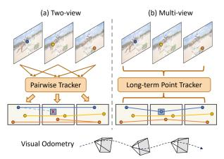
Figure 1. Comparison between two-view approach and multiview approach for visual odometry. (a) In the two-view approach, correspondences are derived for every image pair and concatenated. Managing occlusion becomes challenging without the temporal context. (b) In the multi-view approach, long-term point trajectories can be obtained all at once, enabling the detection of occlusion and tracking points under partial occlusions.
