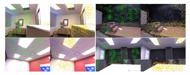
Figure C.4. Visualization of point-wise uncertainty measurements on Replica [28]. Keypoints with the lowest 20% (left) and highest 20% (right) uncertainty are shown in green and yellow, respectively.
