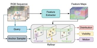
Figure 3. **LEAP Front-end**. Once image feature maps are obtained, selected anchors aid in tracking. The queries and anchors are processed by a refiner to iteratively update states. The model outputs trajectory distribution, visibility, and dynamic track label.
