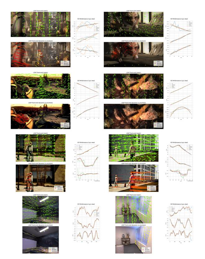
Figure C.1. Qualitative results for Visual Odometry on MPI-Sintel [4], TartanAir-Shibuya [24], and Replica [28]. Upper left: image sample with static (green) point tracking. Lower left: image sample with dynamic (red) and uncertain (yellow) point tracking. Right: comparison with the state-of-the-art VO methods.
