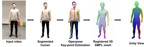
Figure 2. Processing capture video to VR compatible training data
