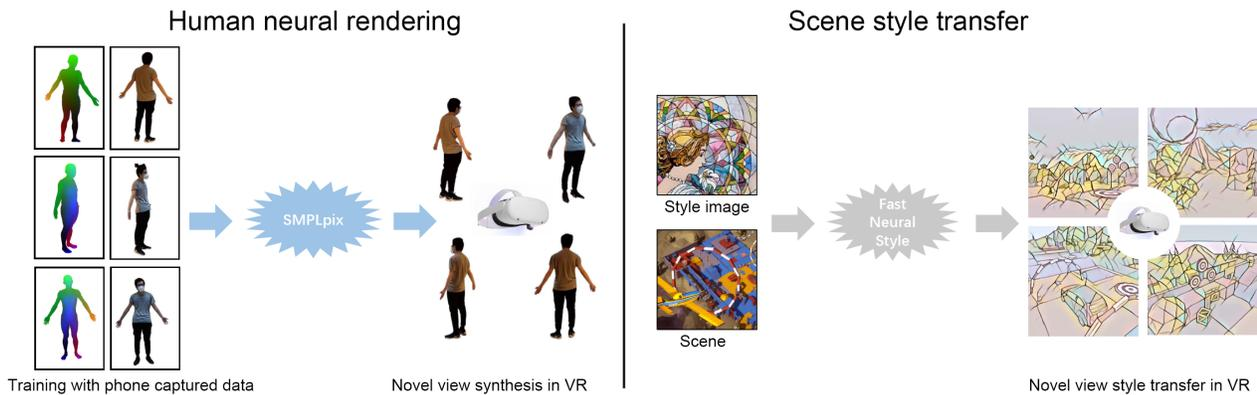
Figure 1. General real-time neural rendering pipeline for VR. Left: human neural rendering. Right: scene style transfer.
